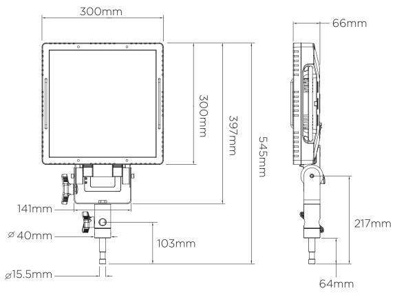
NOTE: Shown with supplied stud adapter installed. This adapter is removable.
